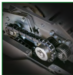
Chain drive with steel gears.
