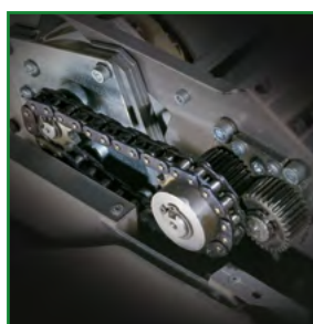
Chain drive with steel gears.
